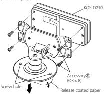
**3** Remove the coated paper from the display stand (Accessory 17), and paste it on the mounting surface. Install the display unit using the screw holes illustrated above when it cannot be secured firmly using the double-sided tape.
