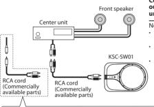
Connect the subwoofer to the subwoofer output (non-fader output) or the RCA jacks for the front output of the center unit.
