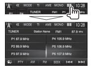
The preset list and the station name for FM Radio Data System (when PS signal is coming in) are displayed.
