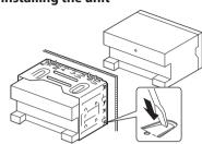
Bend the tabs of the mounting sleeve with a screwdriver or similar utensil and attach it in place.
