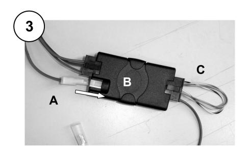
Connect the power lead from Harness A (A(1) Below) into the Yellow (Permanent Power) lead of the Kenwood Harness. Connect the white connector (A(2)) to the vehicle harness.
