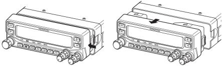
**3** Flip the front panel upside-down, then reattach it to the main body of the transceiver.
