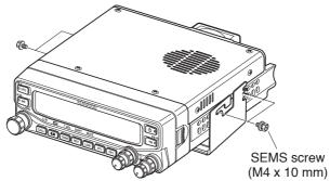
Set an appropriate angle for the main unit, using the 3 screw slots on the rear edge of each bracket side.
