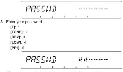
4 After entering up to 6 digits, press the **Tuning** control to set the password.
