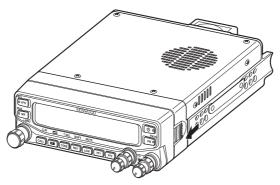
2 Slide the front panel to the left, then pull it away from the main body of the transceiver.
