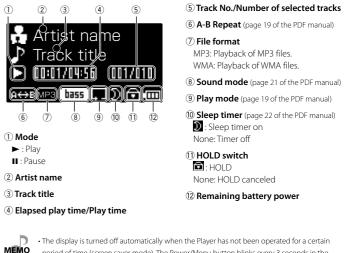
period of time (screen saver mode). The Power/Menu button blinks every 3 seconds in the screen saver mode. The time until the screen saver mode is activated can be changed (page 23 of the PDF manual).
