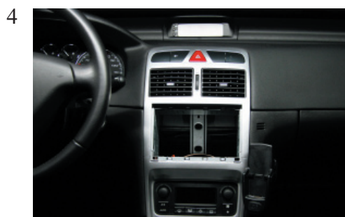
Place the 2-Din metal bracket.
