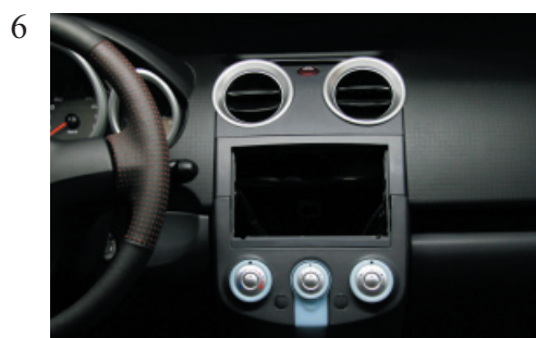
Place the replacement frame and the original dashboard panel.
