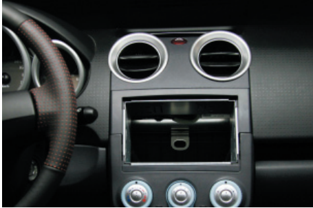
Place the 2-Din metal bracket.
