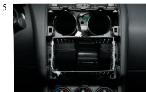
Place the 2-Din metal bracket.
