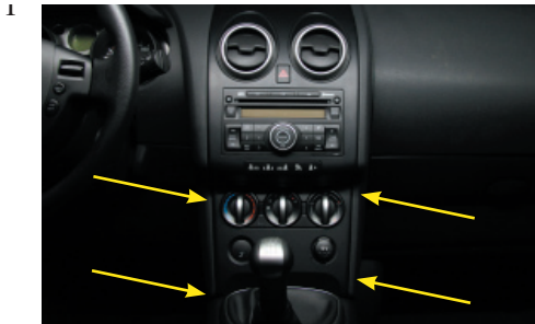
Remove the dashboard panel at the location of the arrows.
