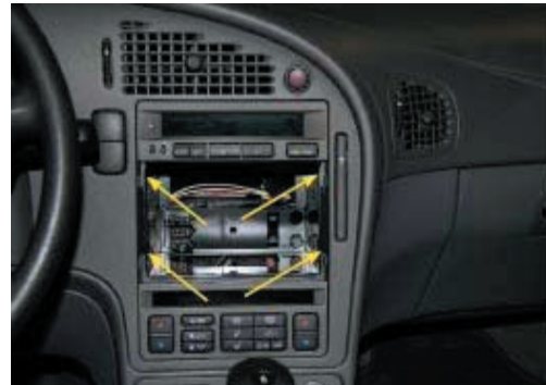
Remove the original radio bracket. At the location of the arrows. On this picture it already has been removed.
