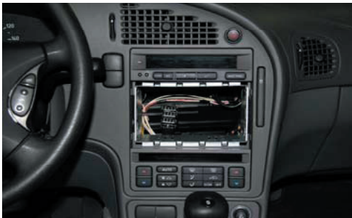
Place the 2-Din metal bracket.
