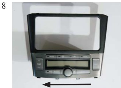
Place the OEM replacement panel on the climate control unit by sliding it to the left .
