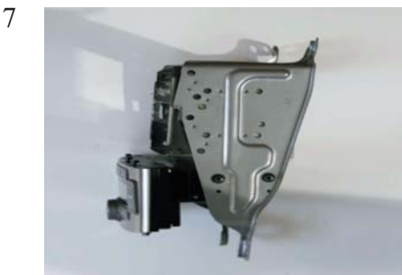
Place the new metal bracket and the climate control unit between the OEM radio brackets. Tighten the climate control with the four original screws.
