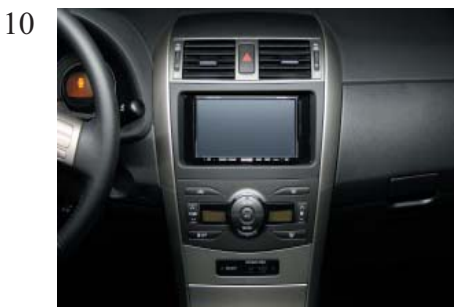
Place the new headunit and replace the dashboard panels in reverse order.
