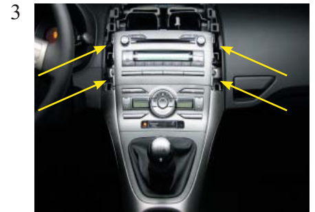
Remove the original radio at the location of the arrows this is tighten by four screws.
