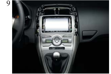
Place the OEM replacement panel.
