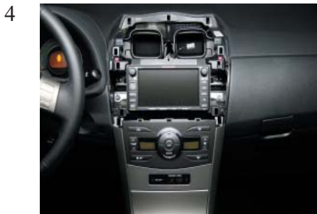
Remove the original radio this is tighten by four screws.
