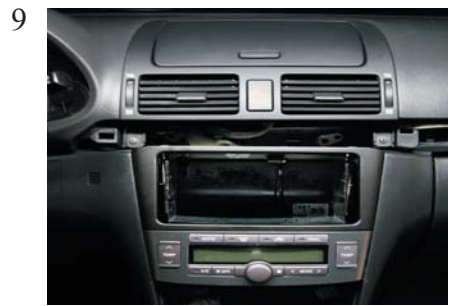
Place the OEM replacement panel with the climate control unit and the metal bracket into the dashboard.
