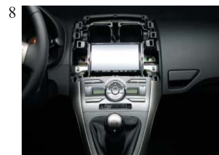
Place the new headunit
