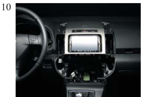
Place the new OEM replacement panel.
