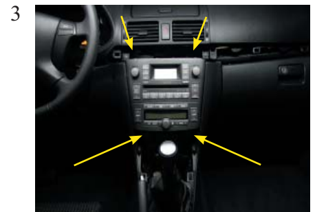
Remove the original radio at the location of the arrows. The radio is tighten by four screws.
