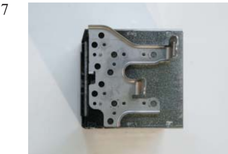
Place the OEM radio brackets on the metal bracket of the new headunit. This will fit in the holes of the metal bracket (if needed mount it with screws).
