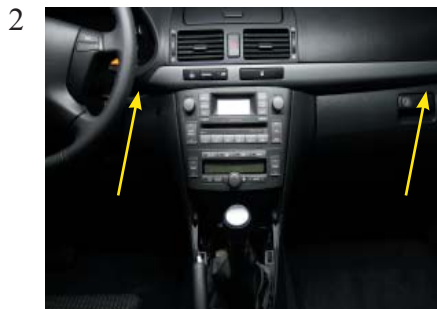
Remove the frame above the radio by using a plastic wedge at the location of the arrows.
