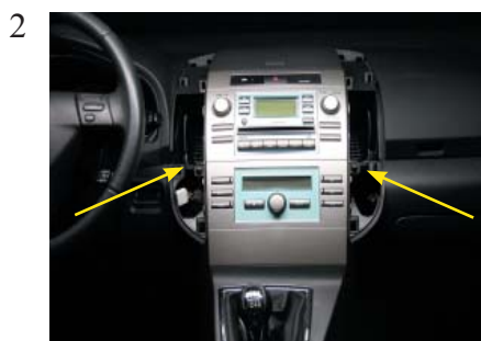
Remove the climate control unit. This is tightened by two screws and pull the unit forwards.
