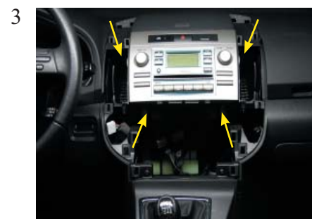
Remove the original radio by removing the four screws at the location of the arrows.
