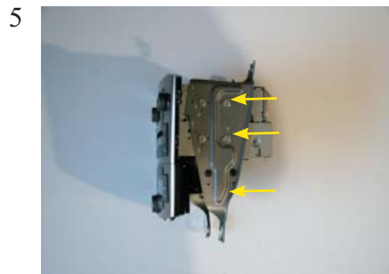
Remove the original OEM metal brackets from the radio and the climate control unit. This is tighten by twelve screws.
