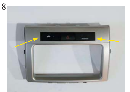
Remove the warning lights switch unit from the original panel and place it in the replacement panel.
