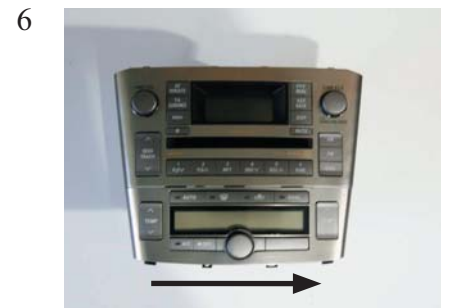
Remove the original radio from the climate control. Slide the climate control unit to the right.
