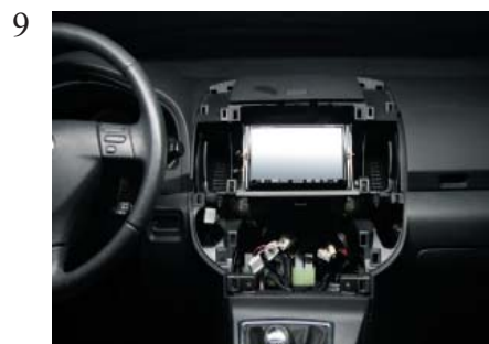
Place the new headunit.
