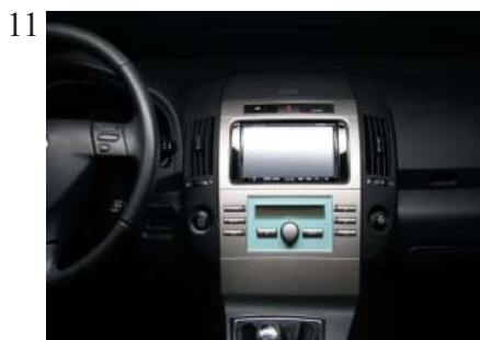
Place the radio trim and replace all dashboard panels in reverse order.
