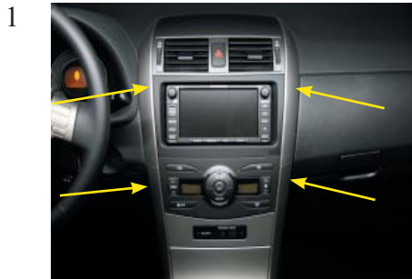
Remove the dashboard panels around the radio at the location of the arrows.
