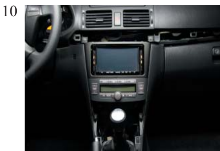
Place the new headunit.
