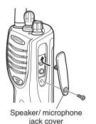
If you are not using a speaker/ microphone, install the cover over the speaker/ microphone jacks using the supplied 3 x 6 mm screw.
