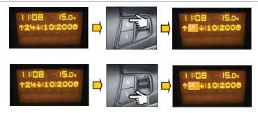
Once the DAY setting is done by pressing the ◀▶ button we will display the MENU DD MM YEAR that is the MONTH setting, by pressing the ◀▶ button again will be displayed DD MM↑YEAR↓ that is the YEAR setting.
