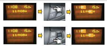
Once the HOUR setting is done by pressing the ◀▶ button will be displayed the MENU voice for the DATE setting∱DD↓ MM YEAR.
