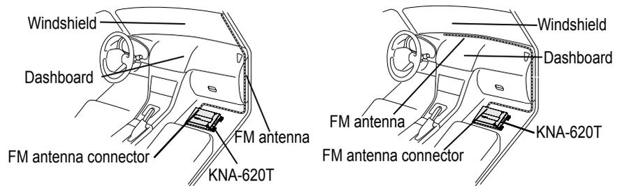
FM Antenna Installed Vertically
