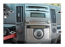
Unclip the air vents on the left and right side of the OEM head unit with a plastic wedge and remove them.
