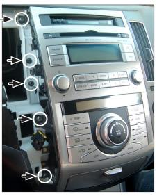
Remove the screws (see arrows) on the left and right side of the OEM head unit
