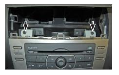
8. Remove the 2 screws at the top of the OEM head unit.
