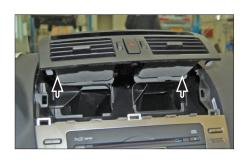
1. Remove the air vent unit above the OEM head unit
