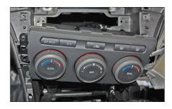
6. Remove the air condition control unit
