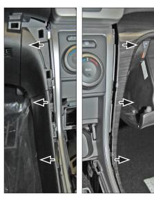
3. Remove the side panels at the left and right side
