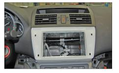
Place the mounting frame at the dashboard. Push the metal frame into the mounting frame. Fix the mounting frame
