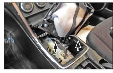
2. Remove the gear shift cover
