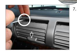
Unclip the air vent unit carefully on both sides with a screw driver.
