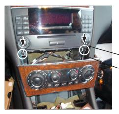
4. Pull out the air condition control unit. Remove the two Torx (TX20) screws under the OEM-Radio.
