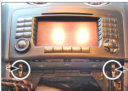
2. Remove the two Torx screws below the OEM head unit.
