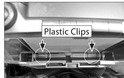
5. Press the 2 plastic clips (see arrows) located under the OEM-Radio.
