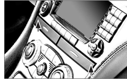
4. Open both cup holders. Remove the 2 Torx TX20 screws (which become visible after removing the centre console)
