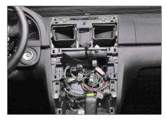
Remove the original bracket. This is tighten by screws.
