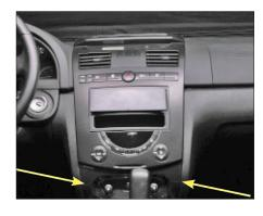
Remove the panel under the climate control panel.
