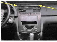
Remove the speaker grill on top of the dashboard. Remove the two which have become visible.
