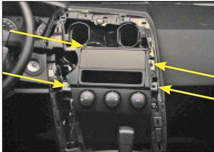
2. Remove the original bracket, which is tightened by four screws at the location of the arrows.
