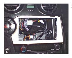
3. Place the new facia plate on the dashboard and fix it with the four screws.
