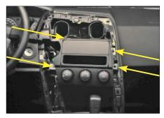
Remove the original bracket, which is fixed by four screws at the location of the arrows.
