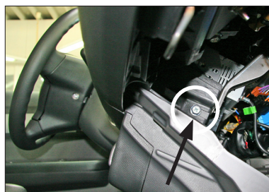
Remove locknut from head unit. (passenger side underneath the dashboard)
