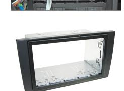
4. Push the metal frame into the facia plate
