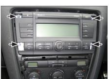
Remove 4 screws fixing the OEM head unit.
