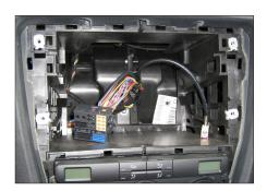
Place mounting frame on the dash board and fix it with the original screws.
