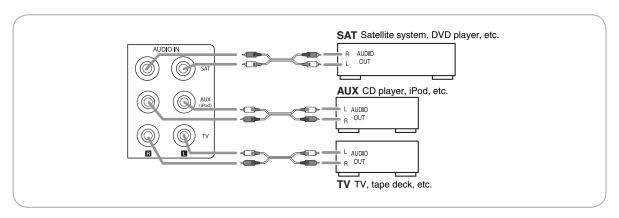
• The AUDIO IN jacks can be connected to the AUDIO OUT jacks of audio or video components.
