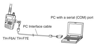
For your information, the following diagram shows how the TH-F6A/ TH-F7E communicates to the PC using a serial (COM) port.
