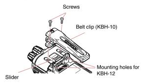
When attaching the optional KBH-12 belt clip, use the mounting holes on the chassis for the KBH-12. (To attach the KBH-12, move the Slider forward.)
