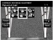
Adjustment is possible by one step to the left and right. If the adjustment is not possible in the currently available range, change the camera position before retrying.
