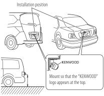
The CMOS-320 should be installed at a height of 50 cm (1.64 feet) or more
