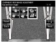
Adjustment is possible by one step up and down. If the adjustment is not possible in the currently available range, change the camera position before retrying.
