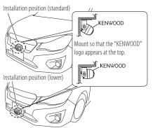
The CMOS-320 should be installed at a height of 30cm to 80cm (0.98feet to 2.62feet)
