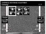
Adjustment is possible by two steps to the left and right. If the adjustment is not possible in the currently available range, change the camera position before retry.
