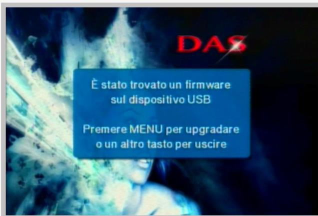
It is **MANDATORY NOT** to turn off the receiver and/or **NOT** to remove the USB key until the update is completed; otherwise the piece will be damaged
