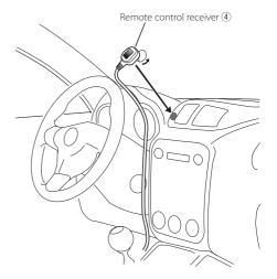
**3** Connect the connectors of the remote control receiver to the main unit.
